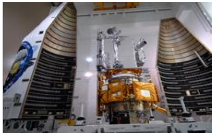
Lunar Reconnaissance Orbiter, or LRO, being prepared for fairing installation. Credit: NASA/Jack Pfaller
